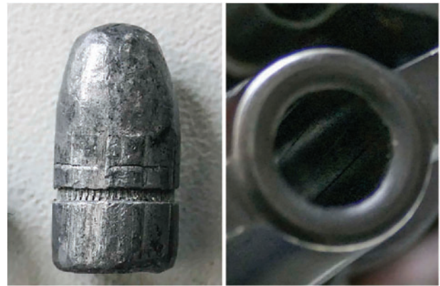
Fig. 6. A cone-shaped projectile (left) and a rifle barrel (right).
