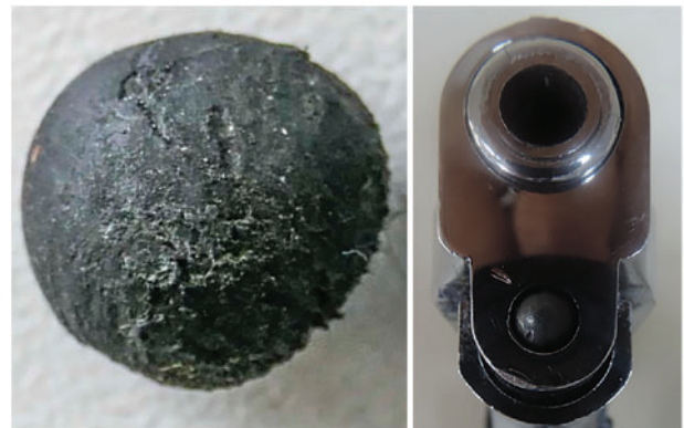
Fig. 7. A rubber bullet (left) and a non-rifled barrel (right).
